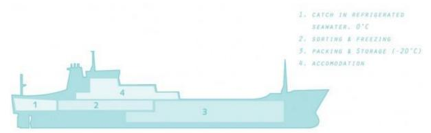
Figure 3.2. Schematic overview of a pelagic freezer trawler
