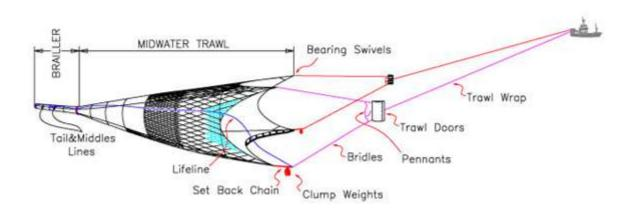
Figure 3.3. Schematic overview of the OTM gear used to fish for small pelagic fish such as Chub mackerel.
