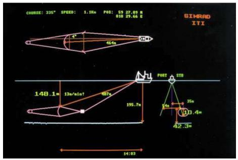
The vessel and net positions can be displayed on plotters and electronic charts. The precision is plus or minus 10 meters for the vessel position,  $\pm 5$  meters for the net position in the display positions, and  $\pm 4$  meters in the net depth (range 2,000 meters: FS 0.2%  $\pm 2$  meters).
