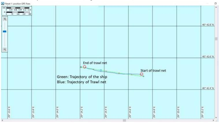
By transforming the ITI data into graphs, it is possible to create a graph that can be used to determine whether a fishing gear has contacted or off the seabed, as shown below.
