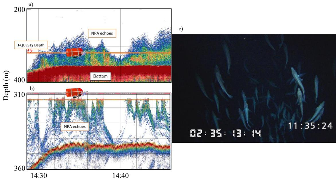
Fig. 1. a) NPA echogram obtained using the hull-mounted quantitative echosounder on the flat top of C-H Seamount in the daytime. Orange solid line indicates the J-QUEST $\chi$  depth. b) NPA echogram obtained using the quantitative echosounder of J-QUEST $\chi$  at 310 m depth. c) Captured NPA school using the stereo video camera and white LED lightings of J-QUEST $\chi$ .
