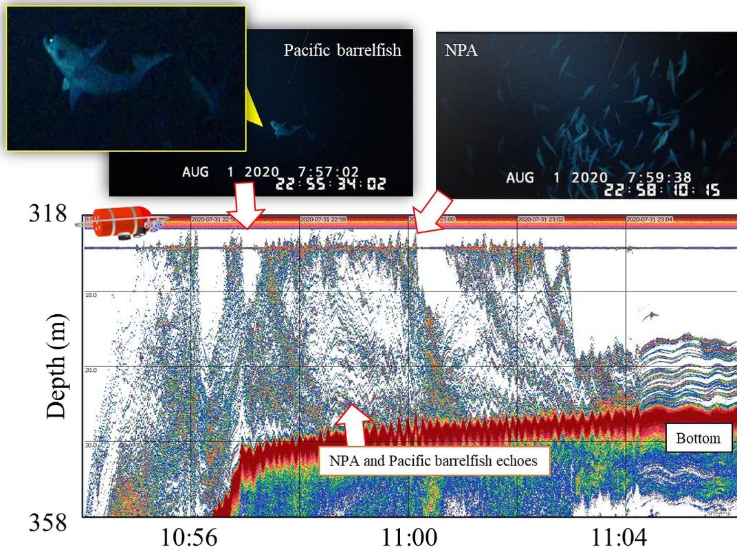
Fig. 4. Echogram that Pacific barrellfish and NPA were mixing obtained using the quantitative echosounder of J-QUEST $\chi$  on the flat top of C-H Seamount in the daytime. their pictures were captured using the stereo video camera and white LED lightings of J-QUEST $\chi$ .
